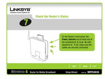
Figure 7-9: Check the Router's Status Screen
